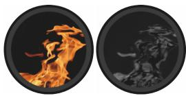
Only when an incident looks like fire visually *and* looks like fire in the infrared spectrum does the FCam signal an alarm condition. This allows the FCam to be extremely sensitive to fire and yet reject almost all false alarms.
